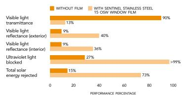
All performance results are based on the film installed on the outside surface of 4mm and 4mm+4mm thick, clear glass.
